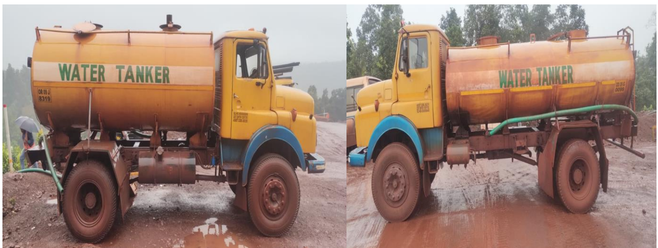
Photo-2 Mobile Water sprinkler tanker for dust suppression.
